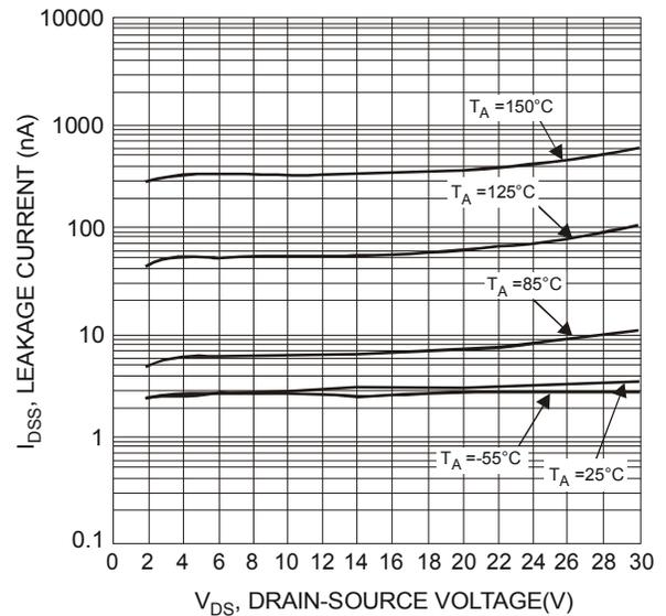
Fig. 10 Typical Drain-Source Leakage Current vs. Voltage
