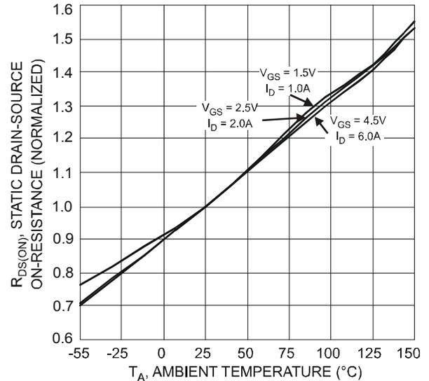
Fig. 4 Normalized Static Drain-Source On-Resistance vs. Ambient Temperature
