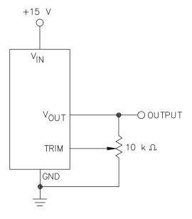
FIGURE 2. V<sub>OUT</sub> trim circuit.
