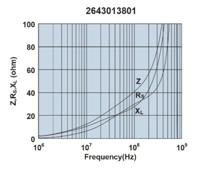
Impedance, reactance, and resistance vs. frequency.
