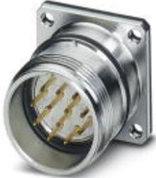
Device connector for front wall, straight, shielded: yes, Screw locking, M23, Number of positions: 16, Type of contact: Male connector, Crimp connection, Flat gasket, 4x Ø3.2
