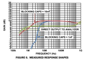
The two upper curves of Figure 6 through the transmission line transformer are emulating the available response at this gain with some added rolloff due to the transformer. These are giving a  $50\Omega$  single ended input to differential output stage that is delivering the equivalent of a 1:3.3 turns ratio step up in gain with a flatness span far exceeding any balun of that turns ratio (1:11 $\Omega$  ratio).
