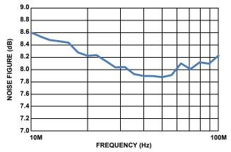
FIGURE 9. MEASURED SPOT NOISE CONVERTED TO A NOISE FIGURE
