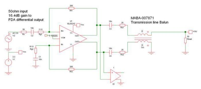
FIGURE 1. ISIM PE SIMULATION CIRCUIT FOR THE DEFAULT CONFIGURATION OF THE ACTIVE BALUN EVM
