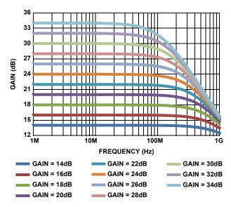
FIGURE 11. PARAMETRIC RESPONSE CURVES FOR  $75\Omega$  INPUT DESIGNS
