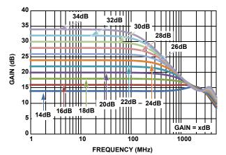
FIGURE 2. RESPONSE CURVES vs Av FOR THE ACTIVE BALUN WITH 50  $\Omega$  INPUT
