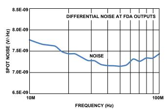
FIGURE 8. MEASURED OUTPUT NOISE FOR THE CIRCUIT OF FIGURE 4
