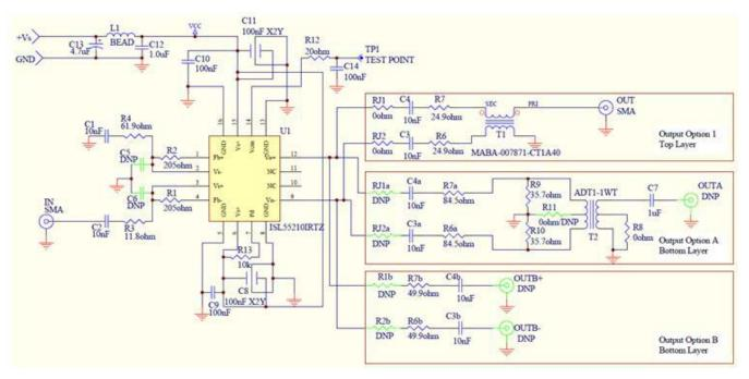
FIGURE 4. FULL BOARD SCHEMATIC
