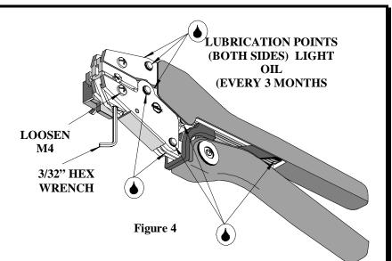
The 64001-0500 (RHT-5765) was engineered for durability, but like any fine piece of equipment it needs cleaning and lubrication for a maximum service life of trouble-free crimping. A light oil, such as 30 weight automotive oil used at the oil points shown in Figure 4, every 5,000 crimps or 3 months will significantly enhance the tool life and ensure a stable calibration.
