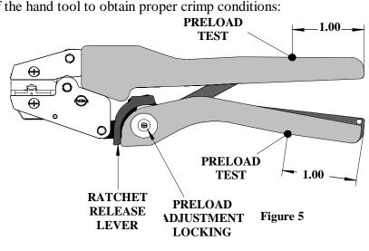
6. Check the crimp specifications after tool handle preload force is adjusted.
