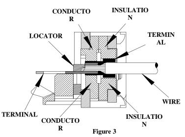
**Note**: Whenever crimping without the locator, make sure the seam of the terminal is oriented up or down in the tool if using unbrazed product, as this will provide higher pull force values.
