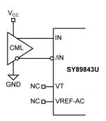
Option: may connect  $V_T$  to  $V_{CC}$ Figure 3c. CML Interface (DC-Coupled)
