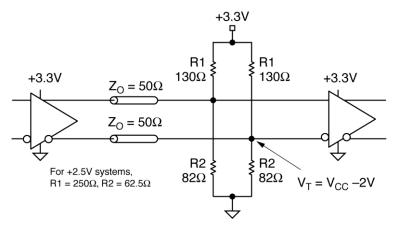
Figure 4a. Parallel Termination-Thevenin Equivalent
