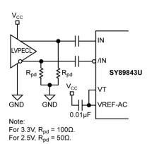
Figure 3b. LVPECL Interface (AC-Coupled)
