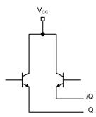
Figure 2b. Simplified LVPECL Output Stage
