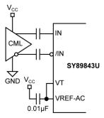
Figure 3d. CML Interface (AC-Coupled)
