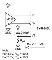
Figure 3a. LVPECL Interface (DC-Coupled)
