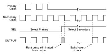
Simplified Example Illustrating RPE (Runt Pulse Elimination)
