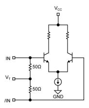
Figure 2a. Simplified Differential Input Stage
