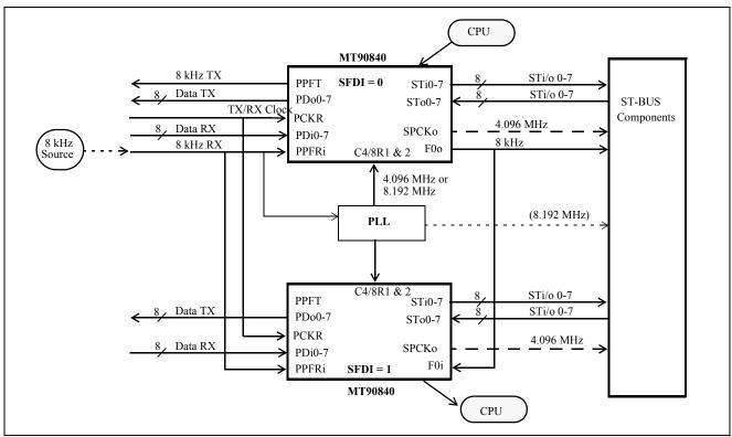
Figure 6b - TM2 Multiple-MT90840 Configuration
