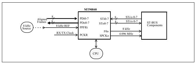
Figure 7 - Timing Mode 3 Configuration
