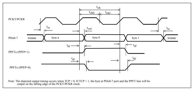
Figure 27 - Parallel Port Transmit Timing (PFDI = 0, PPFT is an output)
