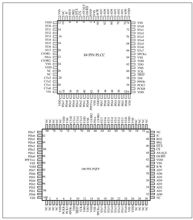
Figure 2 - Pin Connections
