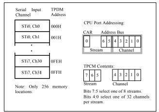
Figure 11a - 2.048 Mbps Balanced Mode TPDM Addressing
