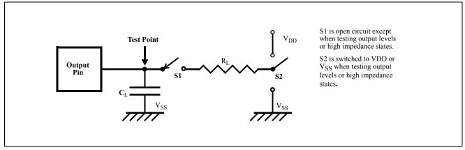
Figure 17 - Output Test Load
