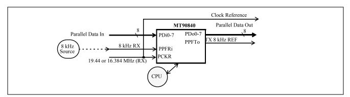
Figure 8 - Timing Mode 4 Configuration
