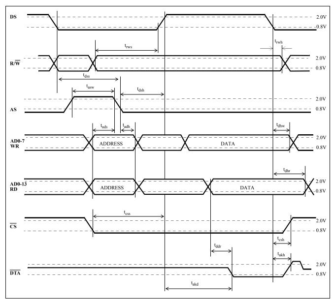
Figure 33 - Motorola Multiplexed Bus Timing
