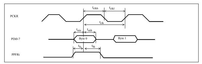
Figure 28 - Parallel Port Receive Timing
