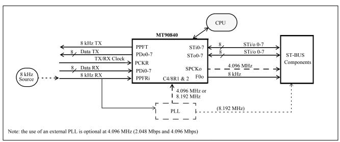
Figure 6a - Timing Mode 2 Configuration
