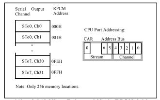
Figure 11b - 2.048 Mbps Balanced Mode RPCM Addressing
