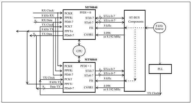
Figure 5b - TM1 Multiple-MT90840 Configuration
