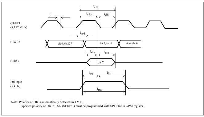
Figure 22 - Serial Port Timing for 8.192 Mbps - TM1 and TM2 (SFDi = 1)
