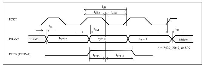
Figure 26 - TM1 Parallel Port Transmit Timing (TM1 & PFDI = 1, PPFT is an input)
