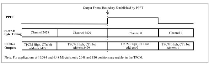
Figure 9 - Parallel Port Control Outputs, CTo0-3
