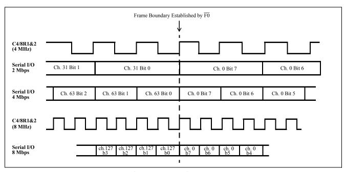
Figure 3 - Serial Port Interface Functional Timing
