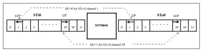
Figure 10 - Balanced Per-Channel Serial Direction Control as Determined by DC Bit
