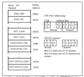
Figure 12a - 2.048 Mbps Add/Drop Mode TPDM Addressing
