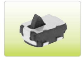
ESE-16 is a one-pole-one-throw, normal-open Detector Switch that comes in a 3.35mm x 2.2mm form factor. It has a body height of 1.5mm and an actuator height of 2.5mm. It can be actuated both vertically and horizontally, at a small actuation force of 250mN max.
