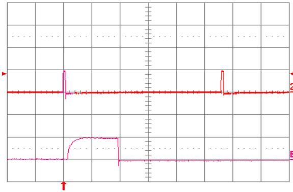
Figure 30. Load current  $I_{out2}$  into a  $10\text{ m}\Omega$  short circuit on  $V_{out2}$  during restart, with  $V_{out1}$  open (no load), at  $V_{in} = 48\text{ V}$ .  $Ch2 = I_{out2}$  (20 A/div, 20 ms/div).  $ChB = I_{out2}$  (20 A/div, 1 ms/div) is an expansion of the on-time portion of  $I_{out2}$ .
