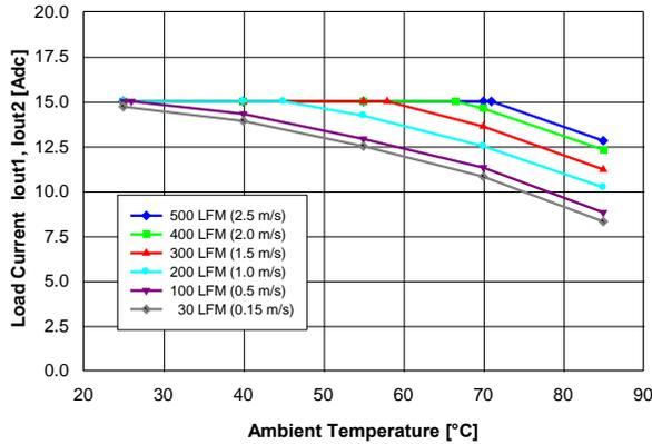
Figure 9. Available balanced load current ( $i_{out1} = i_{out2}$ ) vs. ambient air temperature and airflow rates for converter mounted vertically with  $V_{in} = 48$  V, air flowing from pin 3 to pin 1 and maximum FET temperature  $\leq 120$  °C.
