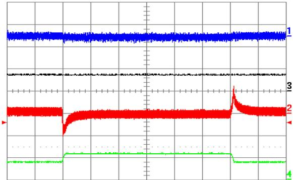
Figure 20. Output voltage response to lout2 load current step-change of 3.75 A (50%-75%-50%) at lout1 = 7.5 A and  $V_{in} = 48\text{ V}$ . Ch1 = Vout1 (50 mV/div), Ch2 = Vout2 (50 mV/div), Ch3 = lout1 (10 A/div.), Ch4 = lout2 (10 A/div.). Current slew rate: 0.1 A/ $\mu\text{s}$ ,  $C_o = 10\text{ }\mu\text{F}$  tantalum + 1  $\mu\text{F}$  ceramic. Time scale: 0.5 ms/div.
