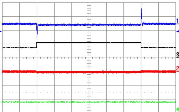
Figure 21. Output voltage response to lout1 load current step-change of 3.75 A (50%-75%-50%) at lout2 = 7.5 A and  $V_{in} = 48\text{ V}$ . Ch1 = Vout1 (100 mV/div), Ch2 = Vout2 (100 mV/div), Ch3 = lout1 (10 A/div.), Ch4 = lout2 (10 A/div.). Current slew rate: 5 A/ $\mu\text{s}$ ,  $C_o = 300\text{ }\mu\text{F}$  tantalum + 1  $\mu\text{F}$  ceramic. Time scale: 0.5 ms/div.
