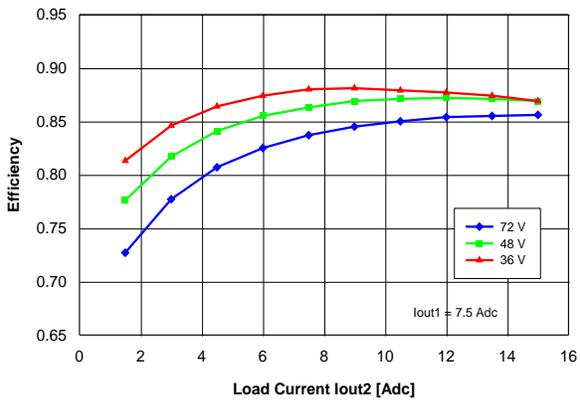
Figure 13. Efficiency vs. load current  $I_{out2}$  and input voltage for converter mounted vertically with air flowing from pin 3 to pin 1 at a rate of 300 LFM (1.5 m/s), for  $I_{out1} = 7.5$  A and  $T_a = 25$  °C.
