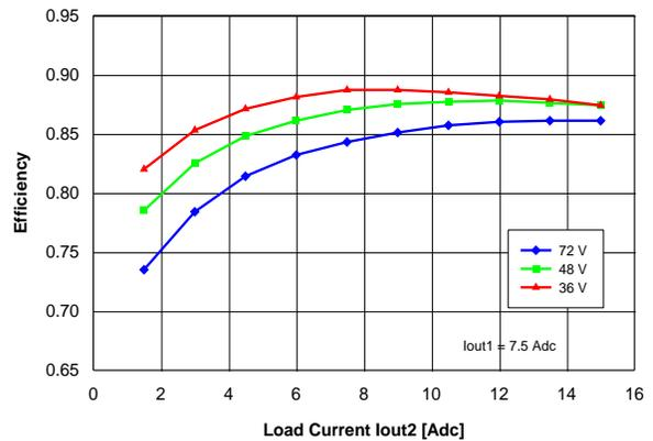
Figure 14. Efficiency vs. load current  $I_{out2}$  and input voltage for converter mounted horizontally with air flowing from pin 3 to pin 4 at a rate of 300 LFM (1.5 m/s), for  $I_{out1} = 7.5$  A and  $T_a = 25$  °C.
