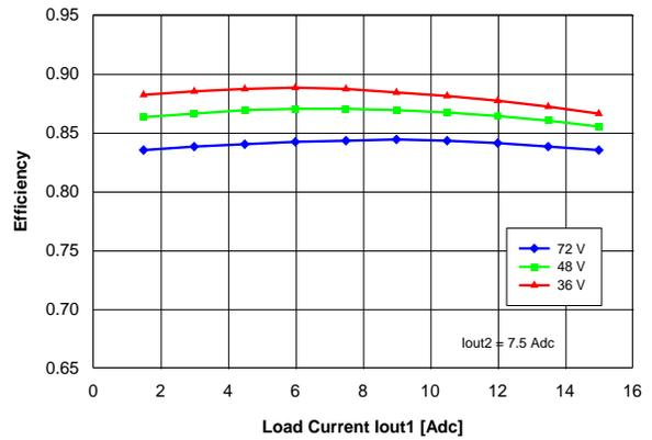
Figure 12. Efficiency vs. load current  $I_{out1}$  and input voltage for converter mounted horizontally with air flowing from pin 3 to pin 4 at a rate of 300 LFM (1.5 m/s), for  $I_{out2} = 7.5$  A and  $T_a = 25$  °C.
