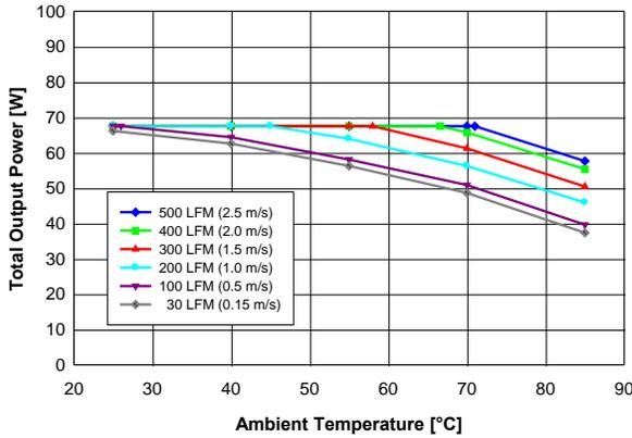
Figure 7. Available output power for balanced load current ( $i_{out1} = i_{out2}$ ) vs. ambient air temperature and airflow rates for converter mounted vertically with  $V_{in} = 48$  V, air flowing from pin 3 to pin 1 and maximum FET temperature  $\leq 120$  °C.
