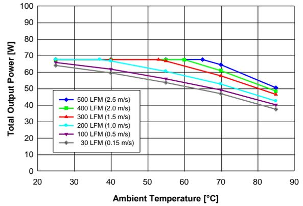
Figure 8. Available output power for balanced load current ( $i_{out1} = i_{out2}$ ) vs. ambient air temperature and airflow rates for converter mounted horizontally with  $V_{in} = 48$  V, air flowing from pin 3 to pin 4 and maximum FET temperature  $\leq 120$  °C.
