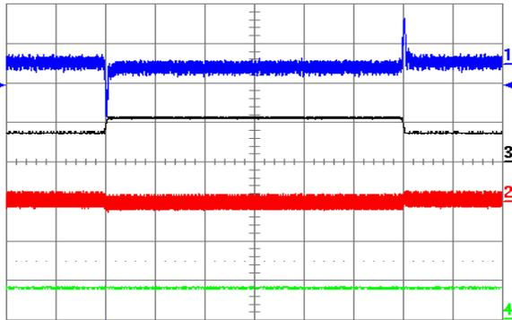
Figure 19. Output voltage response to lout1 load current step-change of 3.75 A (50%-75%-50%) at lout2 = 7.5 A and  $V_{in} = 48\text{ V}$ . Ch1 = Vout1 (50 mV/div), Ch2 = Vout2 (50 mV/div), Ch3 = lout1 (10 A/div.), Ch4 = lout2 (10 A/div.). Current slew rate: 0.1 A/ $\mu\text{s}$ ,  $C_o = 10\text{ }\mu\text{F}$  tantalum + 1  $\mu\text{F}$  ceramic. Time scale: 0.5 ms/div.
