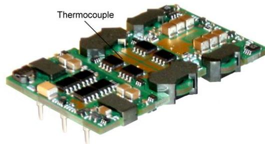
Figure 33. Location of the thermocouple for thermal testing.
