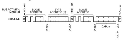
Figure 11. Sequential Read Timing
