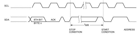
Figure 4. Start/Stop Timing
