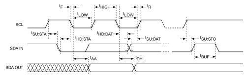
Figure 3. Write Cycle Timing
