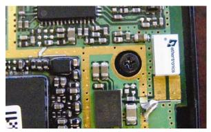
Ethertronics' Savvi series of Isolated Magnetic Dipole™ (IMD) antennas deliver on the key needs of device designers for higher functionality and performance in smaller/thinner designs. These innovative antennas provide compelling advantages for ISM enabled M2M, tracking and smart metering applications.
