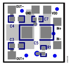
Figure 5. Bottom Layer with Bottom Silkscreen (Mirror Image)
