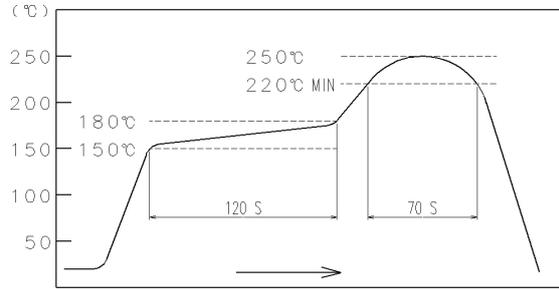
RECOMMENDED PROFILE REFERS TO FIG-2 (TEMPERATURE AT SMT LEAD)
