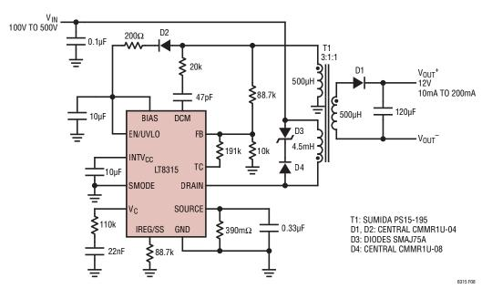
Figure 8. 12V High Input Voltage Isolated Flyback Converter
