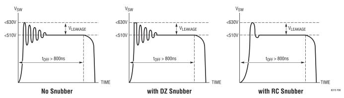
Figure 6. Maximum Voltages for SW Pin Flyback Waveform
