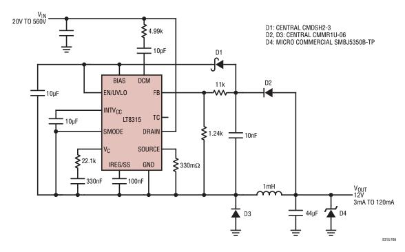
Figure 9. Wide Input Range Non-Isolated 12V Buck Converter
