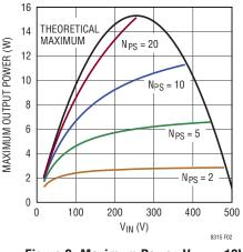
Figure 2. Maximum Power,  $V_{OUT} = 12V$
