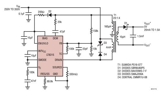
Figure 10. 83% Efficiency 5V/1.5A Isolated Flyback Converter
