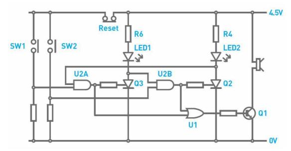
The quiz buzzer is based around two types of logic gates. There are two AND Gates and one OR Gate. Let's first examine Gate U2a. One input of the AND Gate is connected to the Push to Make Switch SW1 on the left of the circuit. These are the switches used by the guiz contestants.
