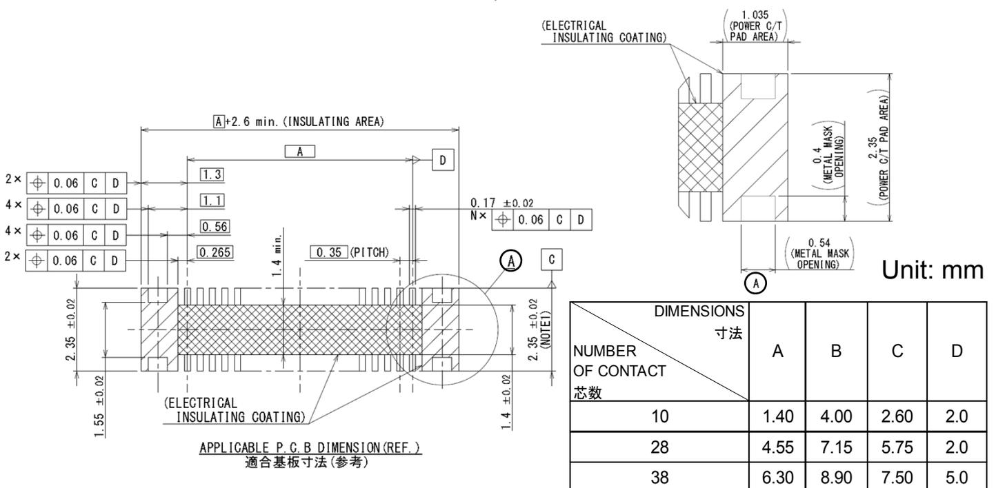
Note 1) Dimension 2.95 ± 0.05 is recommended in case repair is needed.
