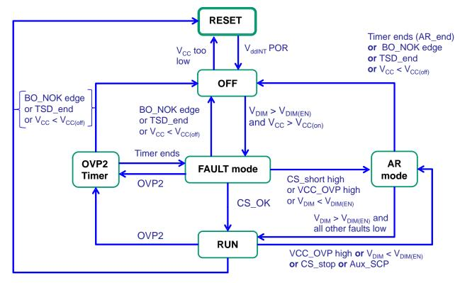
With states: RESET → Controller is dead OFF  $\rightarrow$  Controller is in OFF Mode,  $I_{CC} = I_{CC(off)}$  (50  $\mu$ A max.) **FAULT Mode**  $\rightarrow$  No switching,  $I_{CC} = I_{CC1}$ RUN → Controller is switching AR Mode → the 4-s auto-recovery timer is counting, No switching **OVP2 Timer** → The OVP2 Timer (4-s or 1-s) is counting, No DRV pulses
