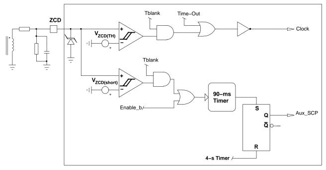
Figure 10. ZCD Block Schematic
