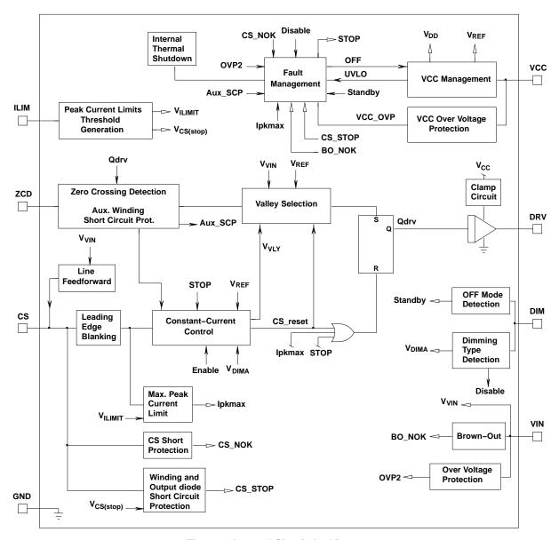
Figure 2. Internal Circuit Architecture
