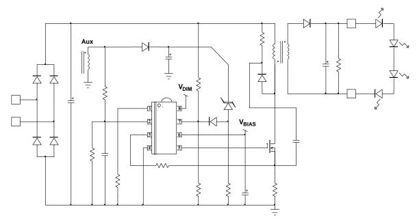
Figure 1. Typical Application Schematic for NCP1370
