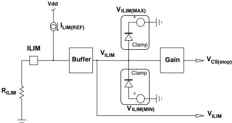
Figure 5. Block Diagram of ILIM Pin
