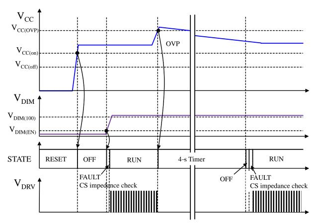
Figure 9. V<sub>CC</sub> Over Voltage Protection Chronograms
