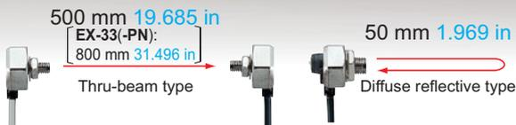
The EX-30 series achieves long distance sensing [thru-beam type: 500 mm 19.685 in (EX-33(-PN): 800 mm 31.496 in), reflective type: 50 mm 1.969 in.]
