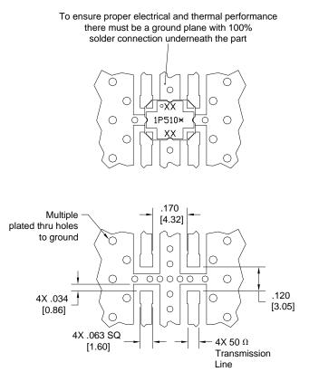
Dimensions are in Inches [Millimeters] 1P510\* Mounting Footprint
