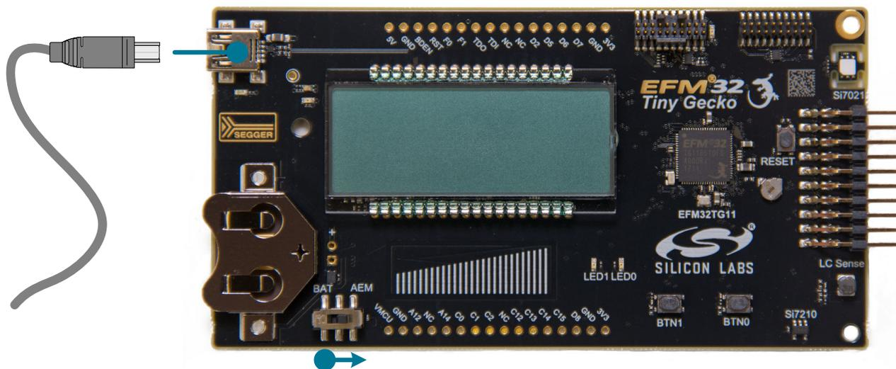
2. The display on the kit will cycle through displaying various information on the segment LCD. To pause the demo on the current screen, press the pushbutton [**BTN1**] on the kit.
