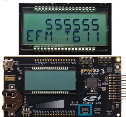
3. Additionally, the display has a feature called charge redistribution, which can be used to reduce the power consumption of the display at the cost of lower display contrast. To enable or disable charge distribution, press the pushbutton [**BTN0**] on the kit.
