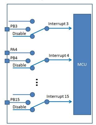
Figure 6 GPIO interrupt multiplexing scheme
