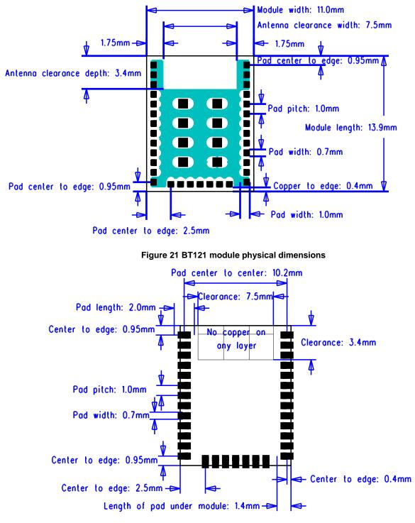
Figure 22 BT121 module recommended PCB pad pattern
