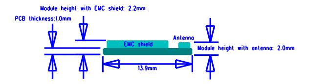
Figure 23 BT121 module side view dimensions
