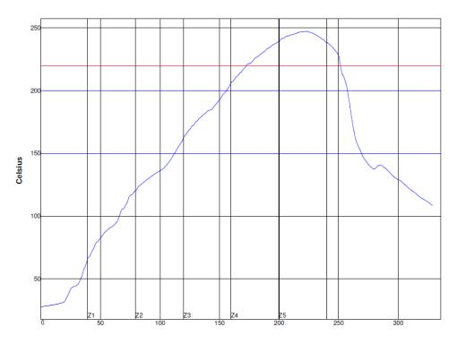
Figure 24 Reference reflow profile example
