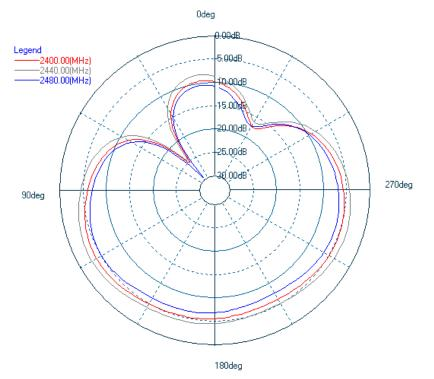
Figure 14 Typical 2D radiation pattern for BT121 with view from above module
