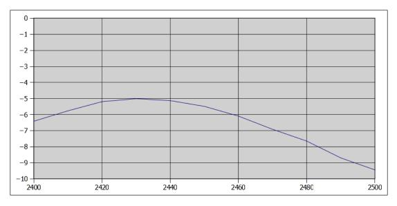
Figure 11 Antenna efficiency related to frequency
