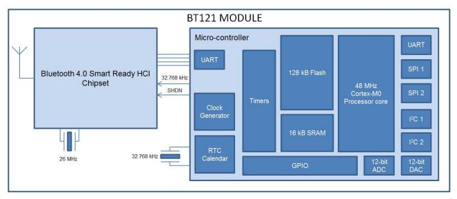
Figure 1 BT121 Bluetooth Smart Ready module block diagram
