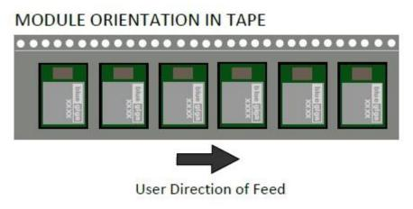
Figure 25 Module orientation in tape and feed direction
