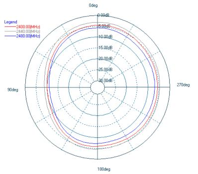
Figure 12 Typical 2D radiation pattern for BT121 with view from module side
