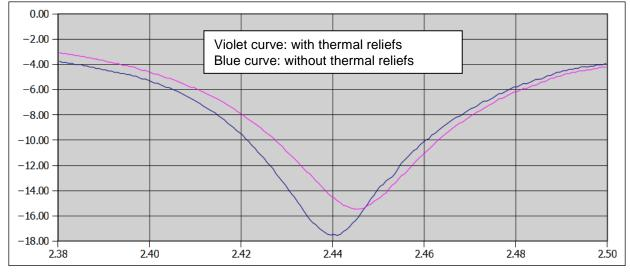
Figure 7 Typical antenna matching
