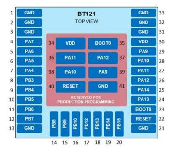
Figure 4 BT121 pin-out (top view)
