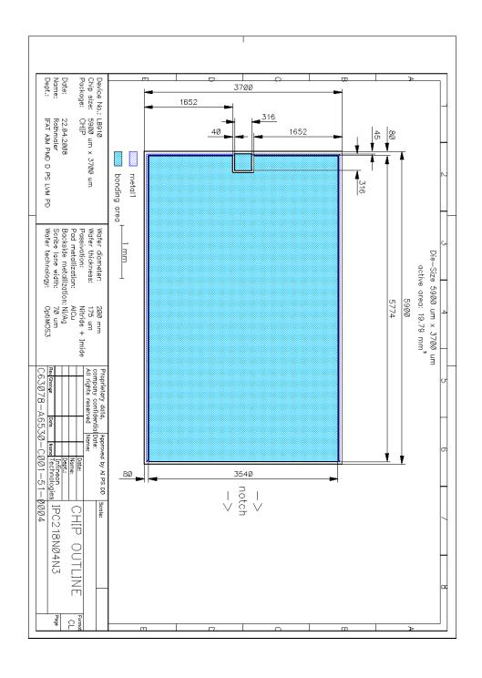
Figure 1 Outline Chip, dimensions in µm
