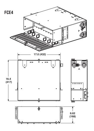
Dimensions are in inches (Dimensions in parenthesis are millimeters)
