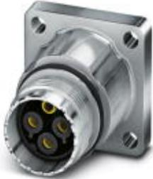
Device connector, front mounting, straight, SPEEDCON locking, M17, Number of positions: 5+PE, Type of contact: Male connector, Crimp connection, Axial O-ring, 4x Ø3.2, shielded: yes, Flange dimensions: 25.75 mm x 25.75 mm
