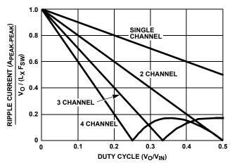
FIGURE 11. RIPPLE CURRENT vs DUTY CYCLE
