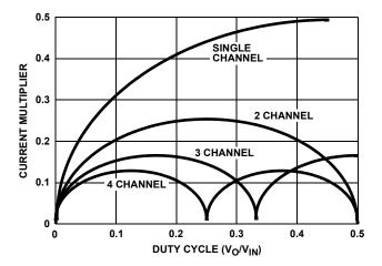
FIGURE 13. CURRENT MULTIPLIER vs DUTY CYCLE
