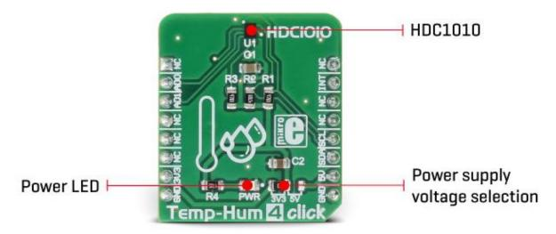
Internally, two sensors are connected to the ADC section, which can be set to sample the measurement with the resolution of 9, 11 or 14 bits, based on the measurement time. OTP memory holds the calibration coefficients that are applied to the measured value and the results are stored on the output registers, in the MSB/LSB format. These values are then used in formulas found in the HDC1010 datasheet so that the final temperature or relative humidity data can be calculated.
