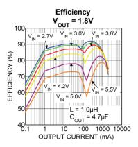
Figure 1. Efficiency Under Load
