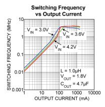
Figure 2. SW Frequency vs. Output Current
