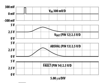
Figure 17. FAULT rejecting a 1  $\mu\text{s}$  , 0 to 2 V to 0 input. Rejection is independent of amplitude.
