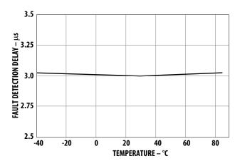
Figure 13.  $\overline{\text{FAULT}}$  detection delay vs. temperature.
