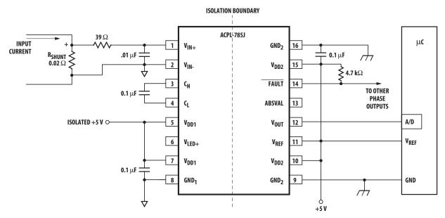
Figure 1. Current sensing circuit.
