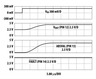
Figure 14. Step response, 0 to 200 mV input, at  $\rm V_{\rm REF}\!=\!5$  V.
