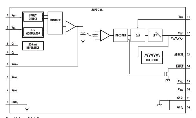
Figure 21. Internal block diagram.
