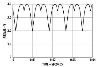
Figure 23. ABSVAL with 2 phases, wired-ORed together.
