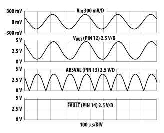
Figure 19. Sine response 400 mV pk to pk 4 kHz input, at  $V_{\rm REF} = 5$  V.
