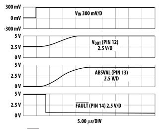
Figure 15.  $\overline{\text{FAULT}}$  detection, 0 to 300 mV input, at  $\text{V}_{\text{\tiny REF}} = 5 \text{ V}.$
