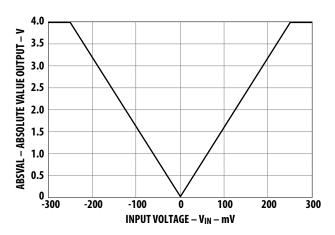
Figure 11. ABSVAL output voltage vs.  $V_{\rm IN}$ .
