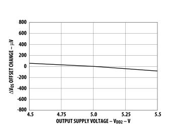
Figure 5. Input offset voltage change vs.  $V_{DD2}$ .
