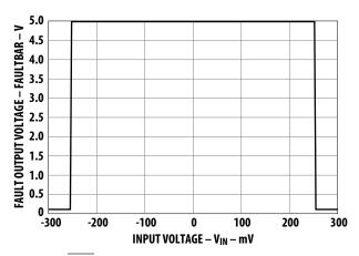
Figure 10. FAULT output voltage vs. V<sub>IN</sub>.
