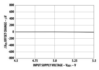
Figure 4. Input offset voltage change vs.  $\mathbf{V}_{\text{DD1}}$ .
