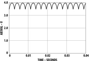
Figure 22. ABSVAL with 3 phases, wired-ORed together.
