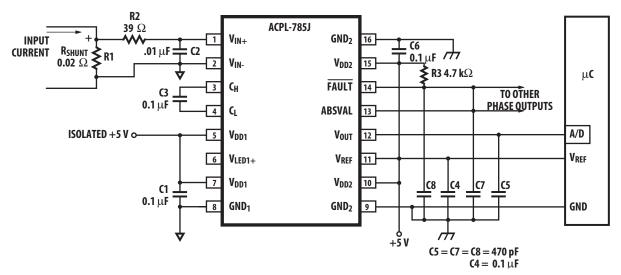
Figure 25. Recommended applications circuit.
