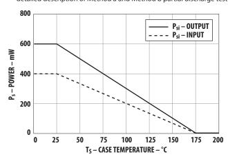
Figure 2. Dependence of safety-limiting values on temperature.
