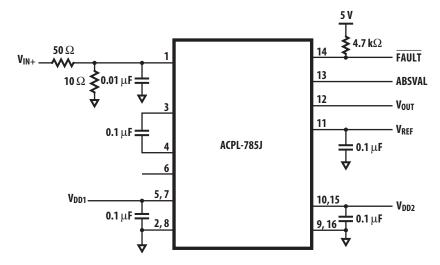
Figure 20. AC test circuit.
