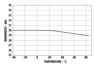
Figure 12. Bandwidth vs. temperature.
