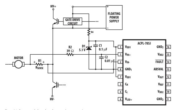
Figure 26. Recommended supply and sense resistor connections.
