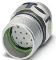
Device connector for front wall, straight, shielded: yes, SPEEDCON locking, M23, No. of pos.: 17, type of contact: Socket, Solder connection, Axial seal, Central fastening M20 x 1.5, can be positioned via a locking nut
