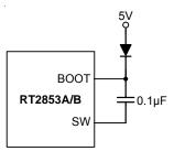
Figure 5. External Bootstrap Diode
