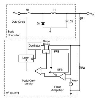
Figure 3. Buck Converter with V<sup>2</sup> Control.
