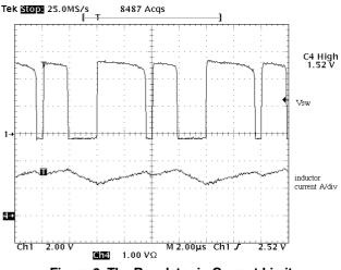
Figure 6. The Regulator in Current Limit
