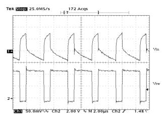
Figure 11. Input Voltage Ripple in a Buck Converter
