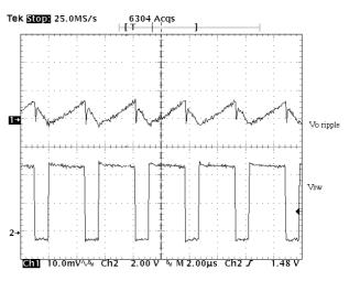
Figure 16. The Output Voltage Ripple Using One 100  $\mu$ F Tantalum Capacitor
