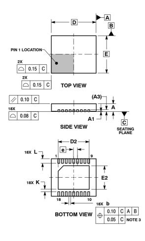
NOTES: 1. DIMENSIONS AND TOLERANCING PER ASME Y14.5M, 1994. 2. DIMENSIONS IN MILLIMETERS.
