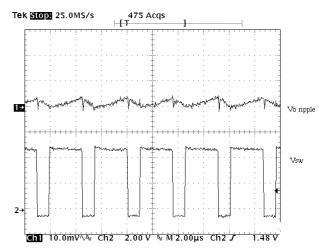
Figure 14. The Output Voltage Ripple Using One 100 µF POSCAP Capacitor
