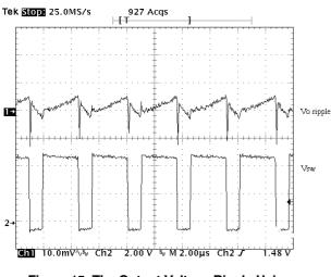
Figure 15. The Output Voltage Ripple Using One 100 µF OS-CON
