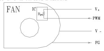
SIGNAL VOLTAGE RANGE:  $0 \sim (V_{+} - 0.5) \text{ VDC}$ HIGH LEVEL
