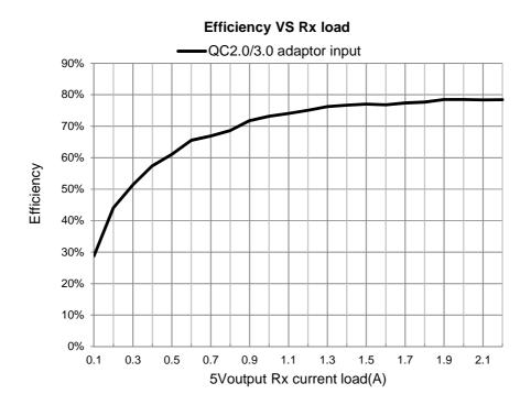
Note: Both results are measured with TSDMRX-5V/10W-EVM.
