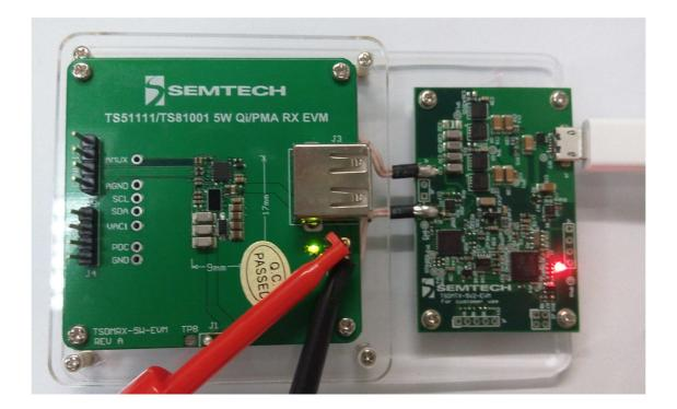
Connect a DC voltmeter across the VOUT+ and VOUT- pins to monitor the voltage being output to the load, and a DC ammeter in series with the VOUT+ line. Set levels to allow for up to 10 volts and 2 amps to be observed.
