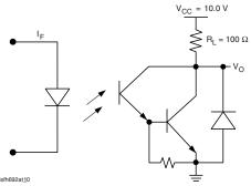
Fig. 1 - Linear Operation (without Saturation)
