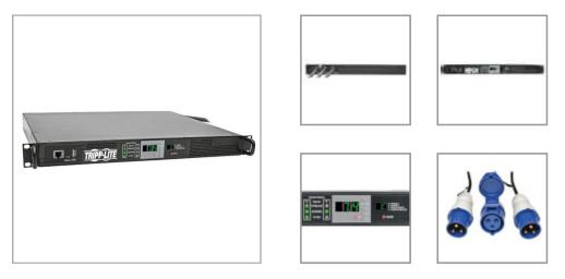
High-capacity 7.4kW PDU with ATS provides remote power monitoring and enables redundant power for non-redundant hardware. Digital display and Ethernet interface allow site power status monitoring for primary and secondary inputs, plus load level monitoring to prevent overload conditions.
