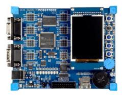
The Keil MCBSTM32EXL Evaluation Boards enable you to create and test working programs based on the STMicroelectronics STM32 family of ARM Cortex™-M3 processor-based devices.
