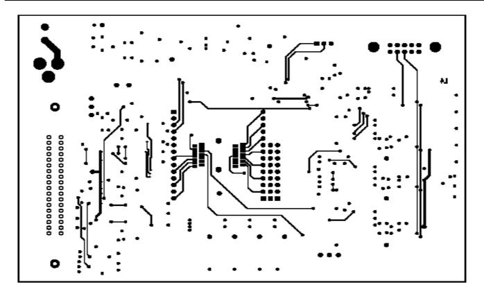
Figure 5. ADM1060 Evaluation Board Layout
