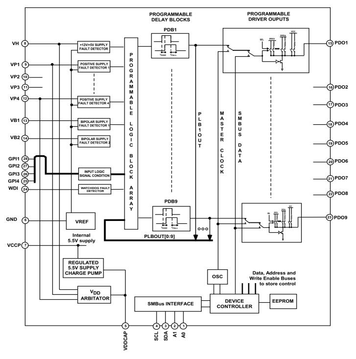
Figure 1. ADM1060 FUNCTIONAL BLOCK DIAGRAM
