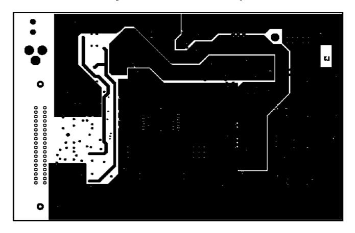
Figure 6. ADM1060 Evaluation Board Ground and Power Planes
