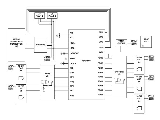
Figure 2. ADM1060 Evaluation Board Block Diagram
