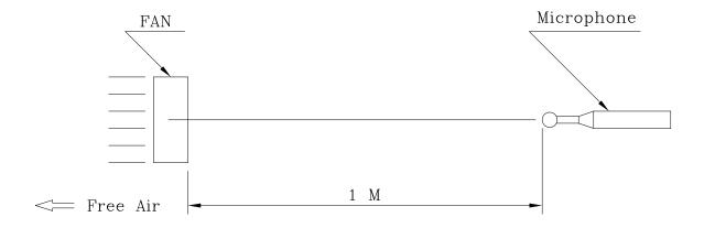
NOISE IS MEASURED AT RATED VOLTAGE IN FREE AIR IN ACOUSTICAL CHAMBER WITH B & K SOUND LEVEL METER.
