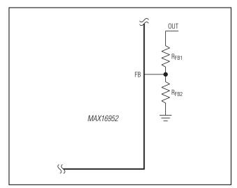
Figure 2. Adjustable Output Voltage
