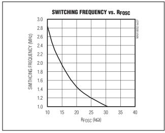
Figure 3. Switching Frequency vs. RFOSC
