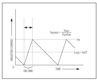
Figure 1. Pulse-Skipping/Discontinuous Crossover Point
