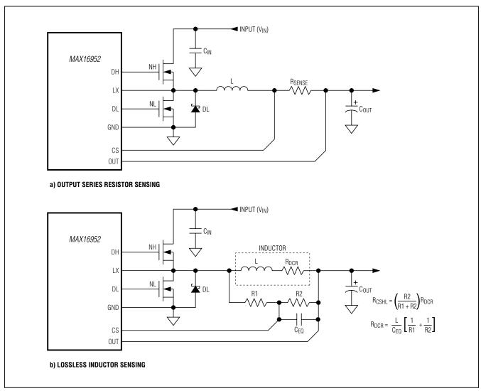
Figure 4. Current-Sense Configurations
