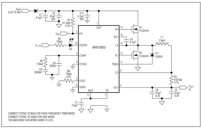
Figure 6. Typical Operating Circuit for Vout = 5V
