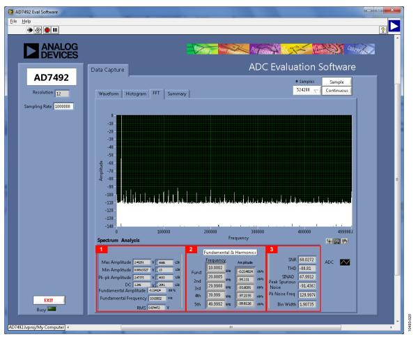
Figure 19. Data Capture/FFT Tab
