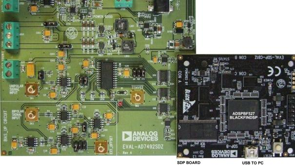
Figure 2. Hardware Configuration, Setting Up the EVAL-AD7492SDZ
