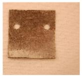
Figure 2: TIM cut for CBM and CSM package types.
