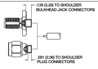
Clean all debris from the prepared cable and insert the cable into the connector, making sure that the cable jacket bottoms out against the internal shoulder of the connector body.
