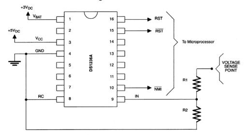
EXAMPLE 1: 5-VOLT SUPPLY, R2 = 10k OHM, V<sub>SENSE</sub> = 4.80 VOLTS
