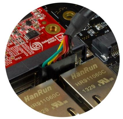
Figure 4 - Connected FTDI cable
