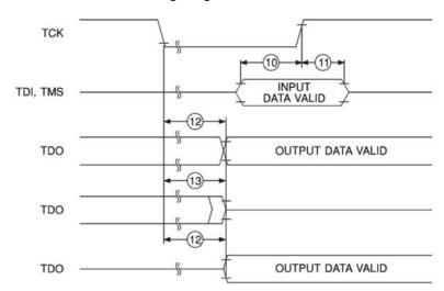
Figure 19. Test Access Port Timing Diagram
