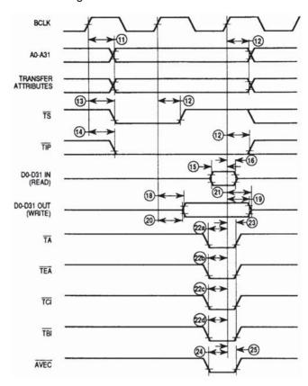
Figure 9. Read/Write Timing
