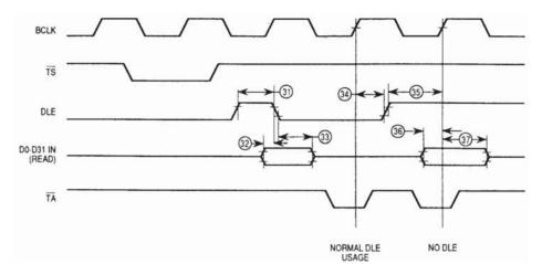
Figure 11. DLE Timing Burst Access
