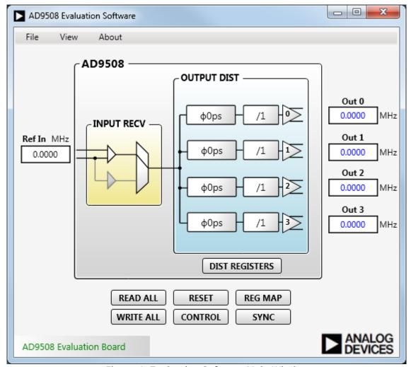
Figure 4. Evaluation Software Main Window
