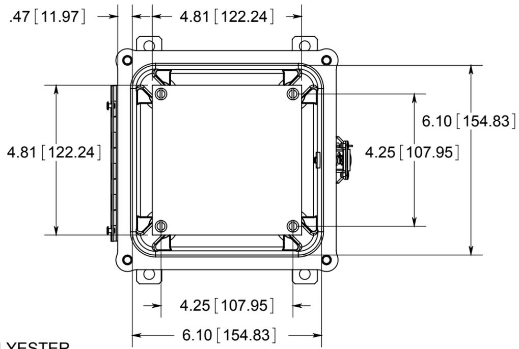
(4) EACH #10-32 BRASS INSERTS AND PLATED CARBON STEEL SCREWS
