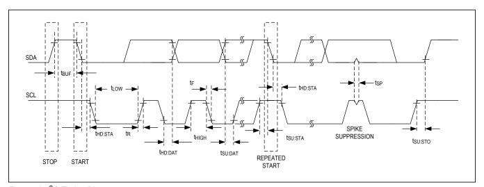
Figure 43: I<sup>2</sup>C Timing Diagram
